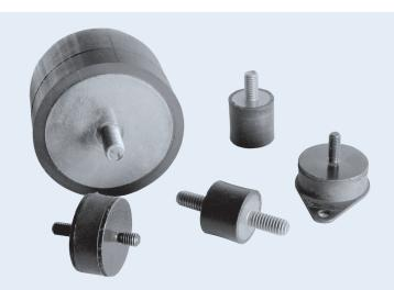
Barry Stud Mounts are designed to support loads up to 260 lbs. per mount in compression and up to 70 lbs. in shear. Their simple design and sturdy construction permit their use in a wide variety of industrial applications. Available in 3 styles: (1) Double stud, (2) Stud/Insert, (3) Bumpers.
